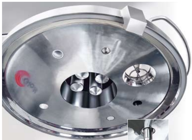
Swivelling lid with inflatable seal, extendible washing nozzles, lamp, metal filter cartridges and sight glass with window wiper
