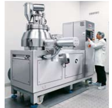
Vertical granulator VG 100, moveable
