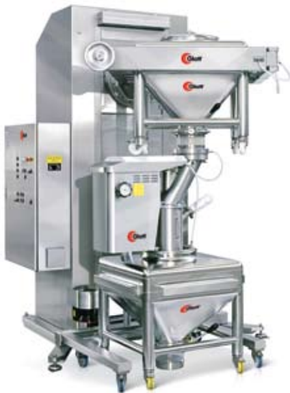
CM 400 container mixer with docked rotor sieve GS 180
