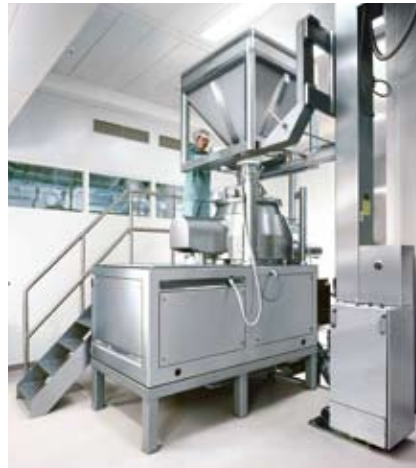
Charging via lifting device L 1500 and container, vertical granulator VG 400
