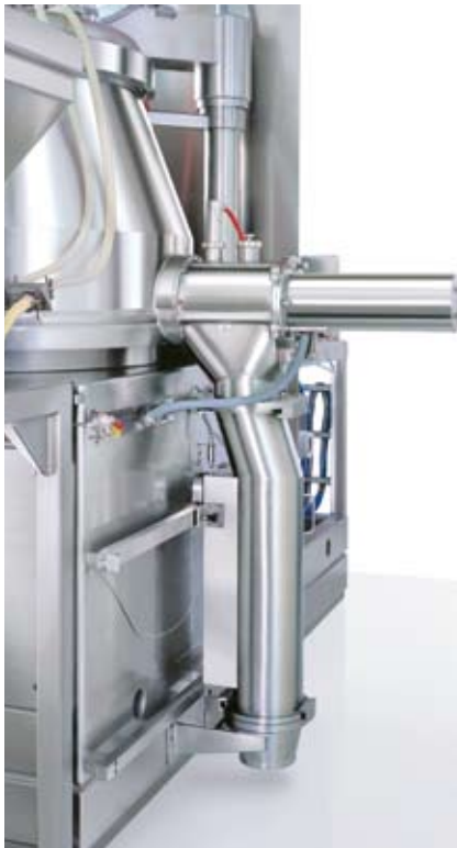
Product discharge with docked bypass tube as an alternative to the wet sieve
