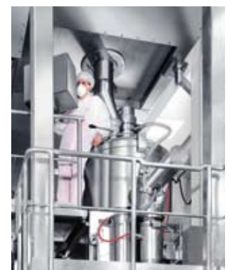
Vertical granulator VG 800 with cylindrical working vessel
