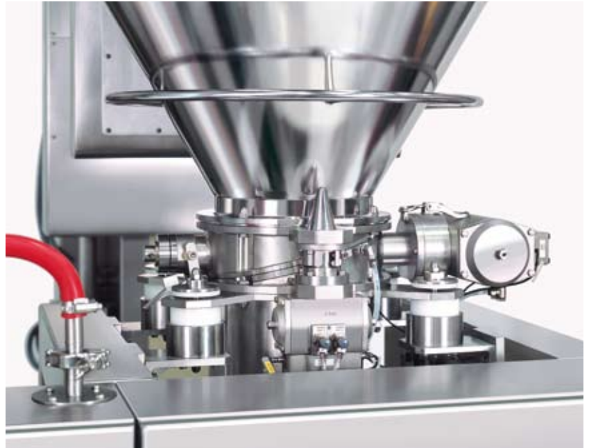
Charging with total containment flap system
